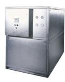
Cooling Technology's DSA Series – a recirculating chiller designed to cool water, brine, glycols and other homogenous fluids – is a self-contained, portable chiller for batch applications, such as dough mixing. It provides fully automated batch delivery of 35°F water that is easily set for various recipes.
